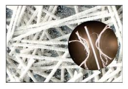
MCI<sup>®</sup> Fibers reduce concrete cracking by 66% and provide corrosion protection to embedded rebars. (Fiber dimensions: 0.015" D and 0.75" L)
